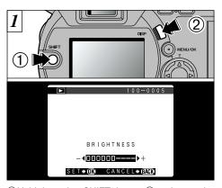
①Hold down the "SHIFT" button ② and press the "DISP" button to display the adjustment bar.
